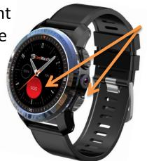
2. Press and hold down the red SOS button on the watch screen OR the bottom right button for 3 seconds
