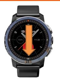
When the watch displays the time, place your finger on the screen and <u>gently swipe</u> from the top of the screen down. The below screen will appear with the Basic Watch Settings
