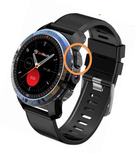
Press and hold down the top right hand button for 3-5 seconds
